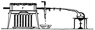
F10. 10.--Method of heating the air (to free it from germs) before introducing it into flasks.
